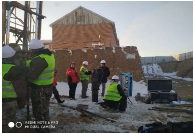
Figure 15. Carrying out pressometric tests
