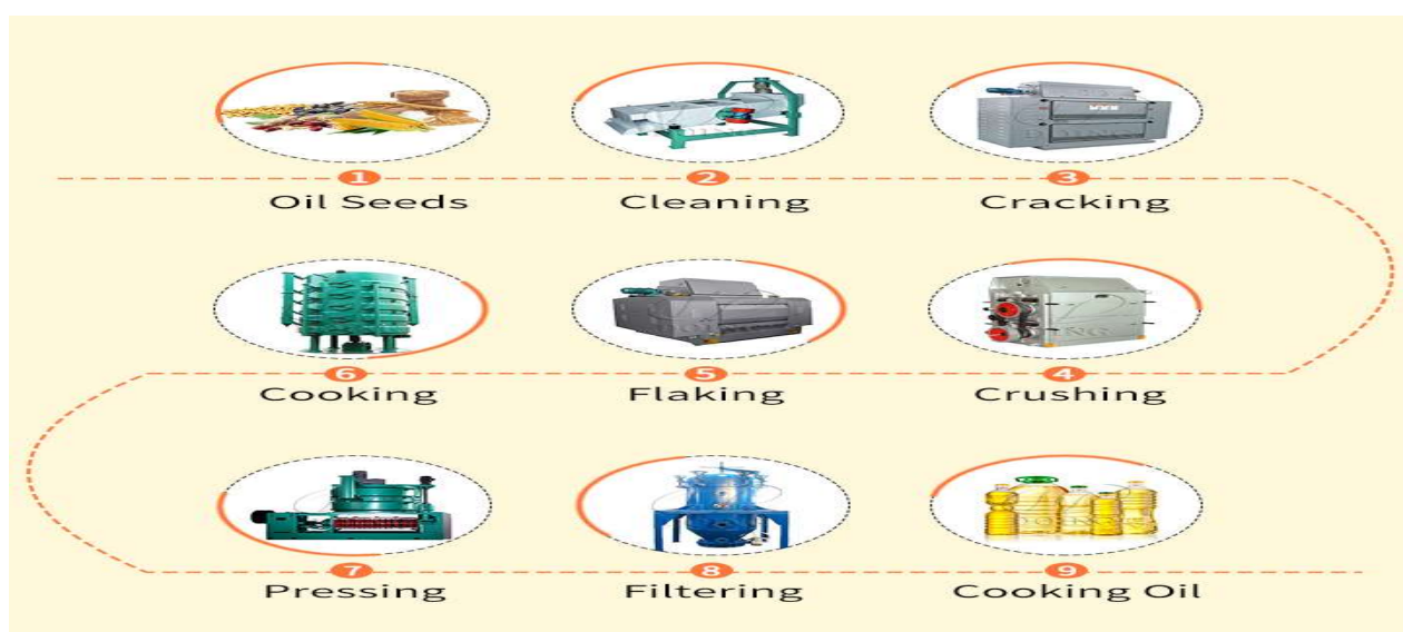
Fig.4. The workflow for obtaining oil from seeds of various plants, which can be implemented using equipment from the Chinese company Henan Glory Oils & Fats Engineering Co. Ltd.
