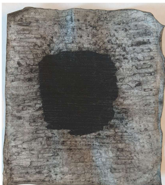
Figure 9. Nafion ® 211 membrane with catalyst layer applied as an ink
