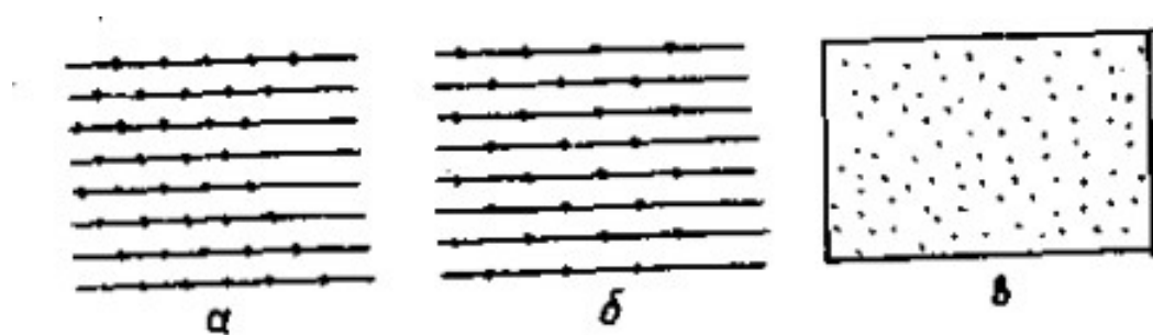
Figure 5 – The system of needle setting in the board a - "herringbone" b - "checkerboard" c - "chaotic"
