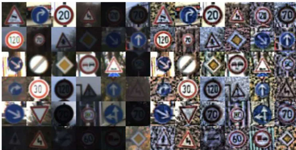
Figure 6: As part of preprocessing for our GTSRB dataset for deep learning classification of traffic signs, we apply a method known as Contrast Limited Adaptive Histogram Equalization (CLAHE) to improve image contrast. Original images input images can be seen on the left — notice how contrast is very low and some signs cannot be recognize. By applying CLAHE ( right ) we can improve image contrast.
