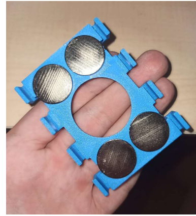
Figure 11 - 3D model driving car on a monorail platform with neodymium magnets
