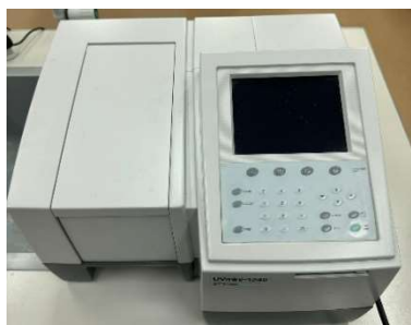
Figure 2- Measuring optical density using a spectrophotometer
