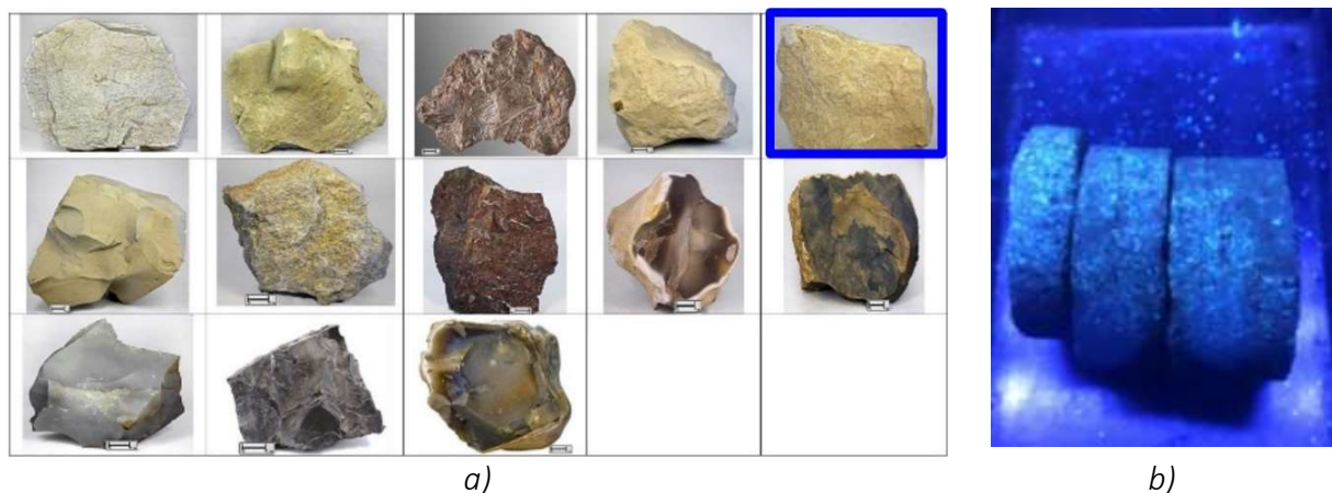
Fig. 4. Photographs of samples from the 10th group of sedimentary (siliceous) rocks (a) and a photograph of a core with fluorescent glow from a depth of 3168 m [1] (b).
