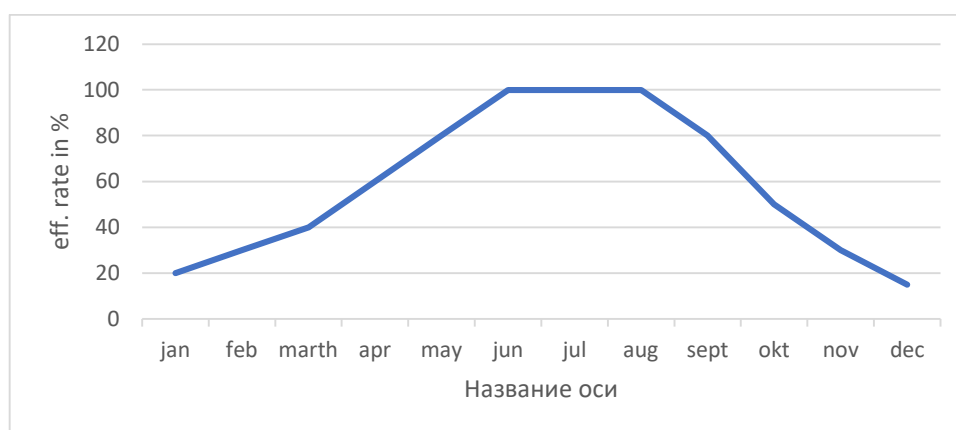
Figure 4 – estimated efficiency of the solar collector (efficiency)
